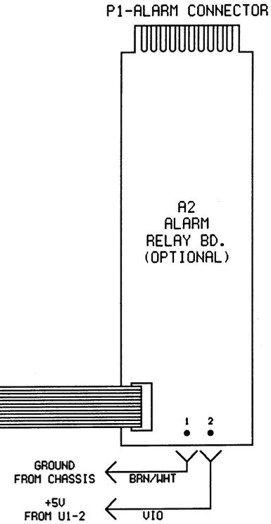
FMM-4A CHASSIS WIRING
