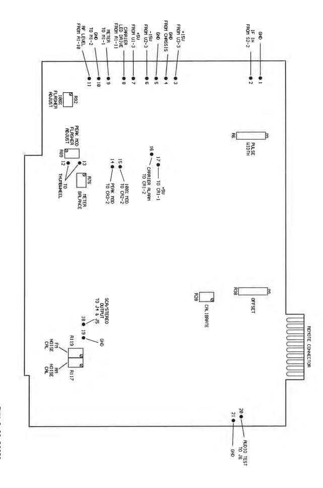
FMM-2 A2 BOARD CONNECTIONS & ADJUSTMENTS BELAR ELECTRONICS
