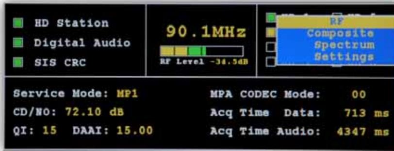
Many of the **FMHD-1** Parameters and Information are accessed using popup menus. To access the popup menus press and hold down the encoder for 2 seconds. To navigate the popup menus rotate the encoder to highlight a menu choice and click the encoder. To exit the popup menu at any time, hold down the encoder for 2 seconds.
