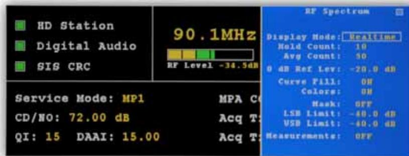
**Display Mode:** The Display Mode affects how the spectrum data is presented, in Real-time mode the spectrum is updated with new data each time, Peak Hold displays the highest value in the last Hold Count value of spectrums, Average displays the average of the last Average Count of spectrums, and Infinite holds the highest values until reset.
