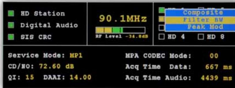
**Filter BW:** Selects Composite filter bandwidth: Stereo + RDS (passes stereo plus 57 kHz RDS), Stereo + 67 KHz (passes stereo thru 67 kHz SCA, and Stereo + 92 kHz (passes stereo thru 92 kHz SCA). To reduce the interference from off-air-noise or HD carriers it is recommended that the Composite filter bandwidth be set as low as possible depending on the SCA's present.
