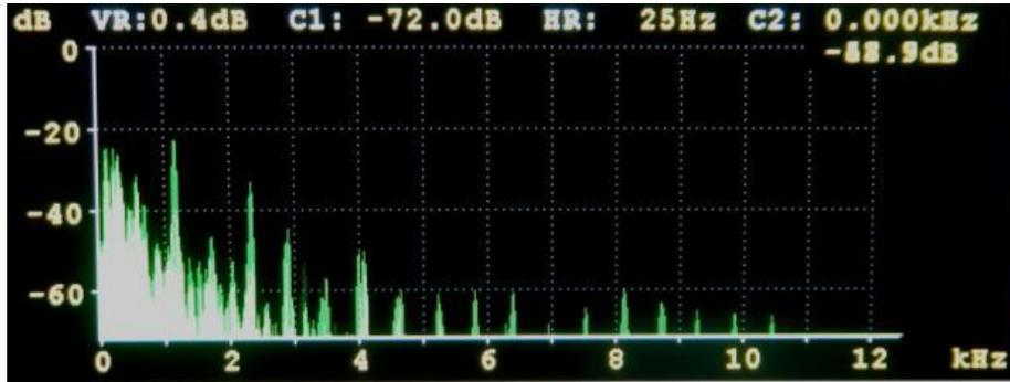
The Audio spectrum screen displays the Audio spectrums from 0 to 24 kHz. The amplitude and frequency scales are both adjustable and have cursors associated with them.
