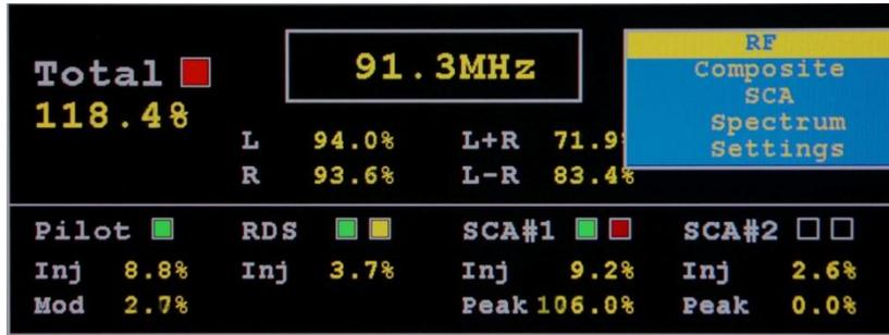
Many of the FMCS-1 Parameters and Information are accessed using popup menus. To access the popup menus press and hold down the encoder for 2 seconds. To navigate the popup menus rotate the encoder to highlight a menu choice and click the encoder. To exit the pop menu at any time, hold down the encoder for 2 seconds.
