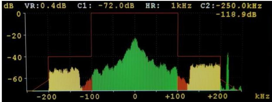
The RF spectrum screen displays the RF spectrum centered around the tuning frequency with frequencies above being positive and below being negative. The amplitude and frequency scales are both adjustable and have cursors associated with them. The RF spectrum is maybe colored such that center green represents the analog carriers, yellow the main HD carriers, and red the extended mode HD carriers.
