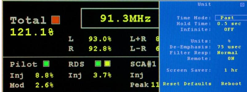
**Time Mode:** The Time Mode affects all the peak modulation readings and bar graphs. In Real Time Mode when a peak exceeds the current displayed peak the value is updated immediately to the new value and held for the Hold Time, until either a new peak is detected or the Hold Time is met. In Past Time Mode, the unit waits the Hold Time and displays the highest peak which was detected during that time period.
