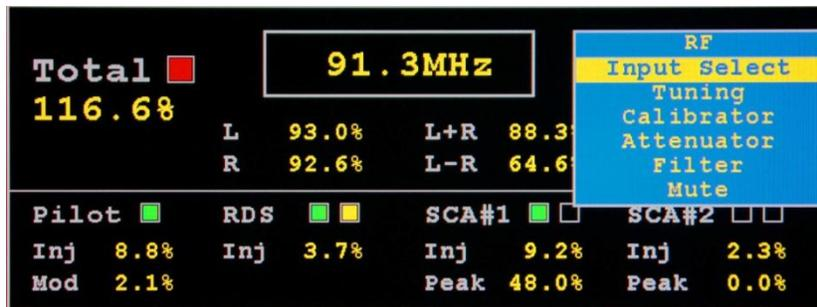
**Input Select:** Select which RF input is used Antenna (off the air) or High Level (tx site).
