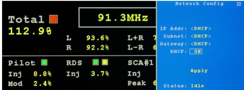
**IP Address:** DHCP must be disabled to enter a static IP
