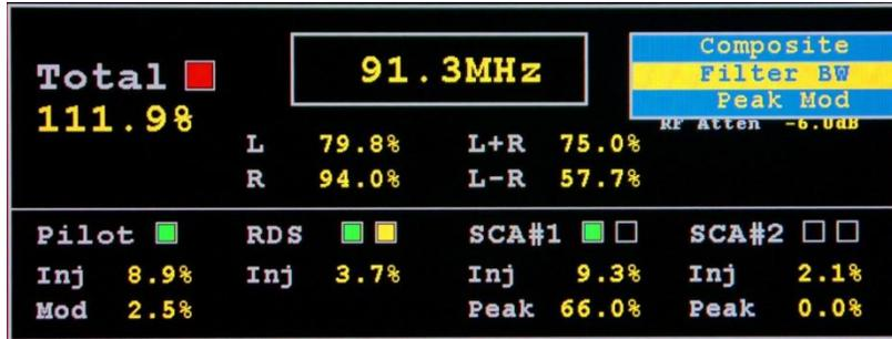
**Filter BW:** Selects Composite filter bandwidth: Stereo + RDS (passes stereo plus 57 kHz RDS), Stereo + 67 KHz (passes stereo thru 67 kHz SCA, and Stereo + 92 kHz (passes stereo thru 92 kHz SCA), and wideband. To reduce the interference from off-air-noise or HD carriers it is recommended that the Composite filter bandwidth be set as low as possible depending on the SCA's present.
