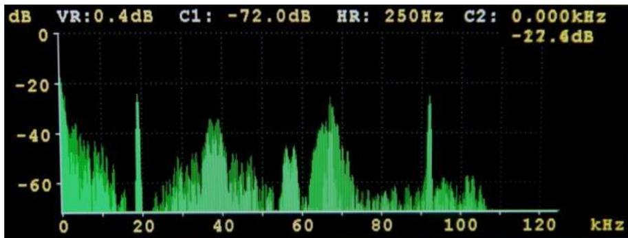
The Composite spectrum screen displays the Composite spectrum from 0 to 150 kHz. The amplitude and frequency scales are both adjustable and have cursors associated with them.
