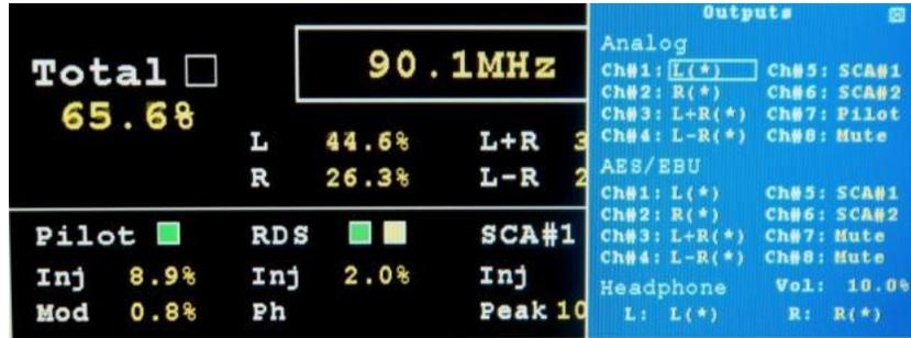
The FMCS-1 provides 8 channels of analog audio output, 8 channels of AES/EBU output, and a headphone output. Any one of these output jacks may be assigned any of the available audio: Mute, L, L(\*), R, R(\*), L+R, L+R(\*), L-R, L-R(\*), SCA#1, SCA#2, Pilot, Test 0dB, Test -3dB, and Test -6dB. The (\*) is the de-emphasized audio, otherwise the audio is flat. The SCA#1 and SCA#2 audio de-emphasis is selected in the SCA pop up window. The Test waveforms are a 1 kHz sine wave at 0, -3, and -6dBFS.
