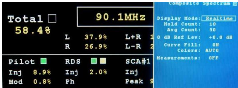
**Display Mode:** The Display Mode affects how the spectrum data is presented, in Realtime mode the spectrum is updated with new data each time, Peak Hold displays the highest value in the last Hold Count value of spectrums, Average displays the average of the last Average Count of spectrums, and Infinite holds the highest values until reset.
