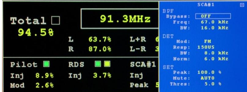
The *FMCS-1* contains two independent SCA decoders SCA#1 and SCA#2. The parameters and setup of these decoders are the same so only one will be described.
