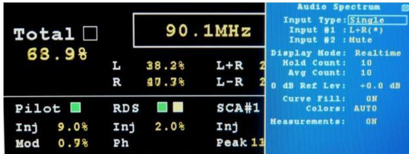
**Input Type:** Selects a single or dual input spectrum.
