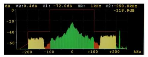
The RF spectrum screen displays the RF spectrum centered around the tuning frequency with frequencies above being positive and below being negative. The amplitude and frequency scales are both adjustable and have cursors associated with them. The RF spectrum is maybe colored such that center green represents the analog carriers, yellow the main HD carriers, and red the extended mode HD carriers.
