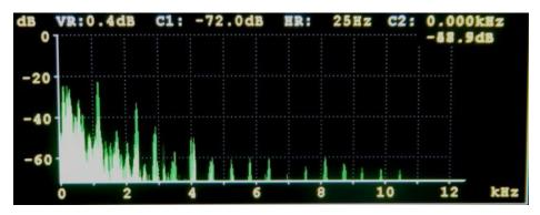
The Audio spectrum screen displays the Audio spectrums from 0 to 24 kHz. The amplitude and frequency scales are both adjustable and have cursors associated with them.
